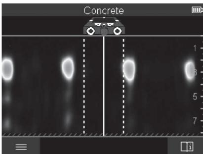
The **<Signal View 2D>** indicates the signal strength at each measuring point in combination with the object depth. The **<Signal View 2D>** is a variant of the **<Object View>**. It displays signal strengths instead of object symbols. The maximum signal strength represents the upper edge of the objects.
