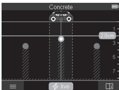
The <Object View> offers the best possible measuring results and the maximum measuring depths. The detected objects are displayed over the measuring path with depth information and, if available, with material properties.
