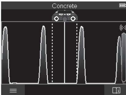
The **<Signal View>** displays the signal strength at each measuring point without information on the object depth.
