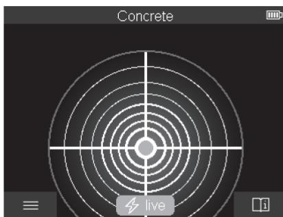
In the <**Spot View**>, a first measuring result is already displayed without moving the measuring tool over the substrate. It is therefore particularly suitable for measurements in corners or narrow places. The maximum measuring depth is 6 cm. Objects found are displayed with material properties, if available, but without depth information.
