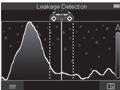
In this measuring mode, the relative material moisture of the surface is displayed. It is therefore suitable for locating the point of maximum material moisture and thus a possible leakage.
