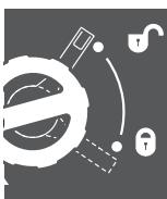
Indicates the position of the locking lever for locking the saw blade and for adjusting the bevel angle (saw blade tiltable).
