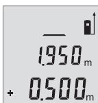
Press button **6** to add measured values or press button **3** to subtract measured values. "+" or "-" will appear at the bottom of the display. Take another measurement. The current measured value will be shown at the bottom of the display, and the previous measured value will be shown above it.
