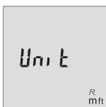
Hold down the On/Off button **5**. When the required unit of measure is displayed, let go of the On/Off button **5**. After releasing, the measuring tool switches itself on with the selected setting.
