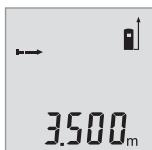
Move the measuring tool until the required distance value is indicated in the bottom of the display.
