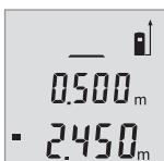
Press button **6** to add measured values or press button **3** to subtract measured values. The result will be shown at the bottom of the display after “=”, and the current measured value will be shown above it.
