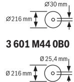
The saw blade diameter must match the information specified on the symbol.
